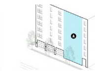
Example of large blank wall area between fenestration elements.
