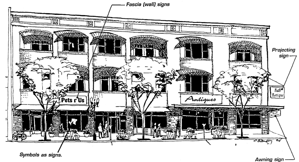
Figure 11: Different types of signs can be integrated with the building's facade to be consistent with one another.
