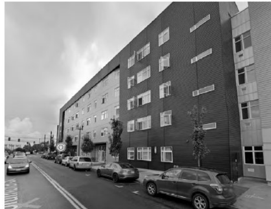
DON'T: Create buildings with long flat facades. Design buildings to have modulations that reflect a residential rhythm and pattern.
