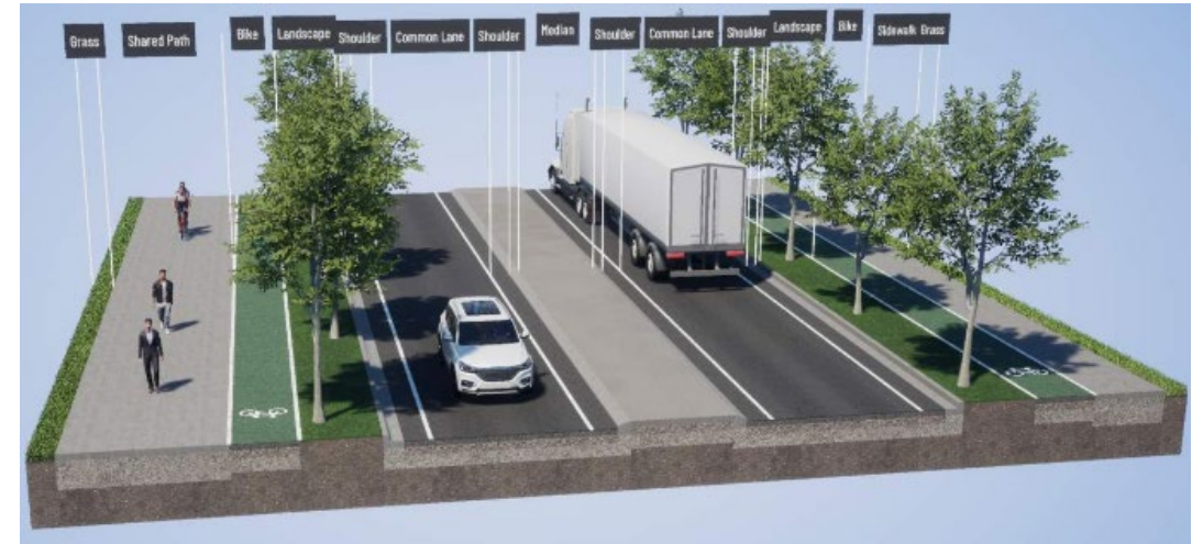
B - Shared Use Path One Side with Cycle Tracks on Both Sides
