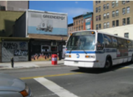
Recessed stop bars allow larger vehicles to make right turns. Photo: Nelson\Nygaard
