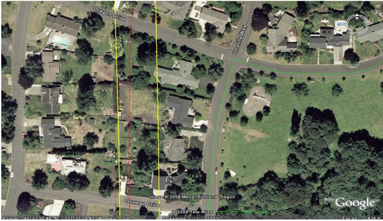
High Voltage Transmission Line – Oswego Drive to Oregon Drive Yellow lines indicate 100 Foot Easement and Red is Transmission Line
