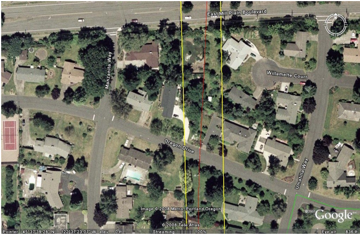
High Voltage Transmission Line – Oregon Drive to Mill Plain Boulevard Yellow lines indicate 100 Foot Easement and Red is Transmission Line
