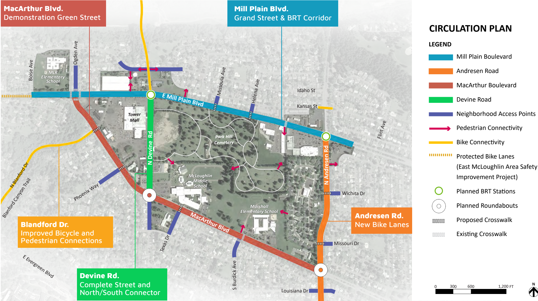
Fig 20: Proposed Access and Circulation Improvements
