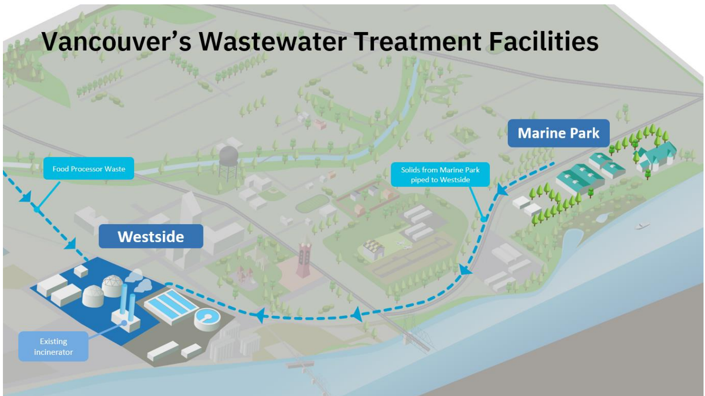
Figure 1 All wastewater solids are piped to Westside for treatment. Current treatment is incineration at Westside and trucking ash to landfill.
