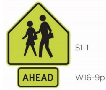
Figure 6 Crossing Warning Assembly
