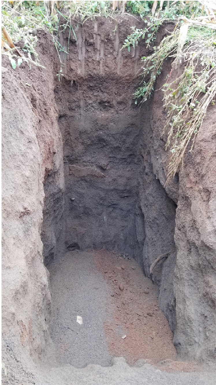
Typical Test Pit Profile, Test Pit TP-4
