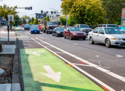
Vertical separation allows trucks and vulnerable users to co-exist. Photo: City of Vancouver
